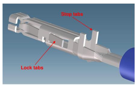
Ensure terminals are fully seated and locked during terminal insertion to the receptacle housing
