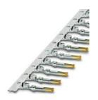
Crimp contact, Socket, rolled, Taped articles, number of pieces per reel: 500, contact diameter: 1 mm, crimp range:  $0.22~\text{mm}^2$  ...  $0.56~\text{mm}^2$ , Item is lead-free in accordance with RoHS II without Exemption 6c (Pb <0.1%)
