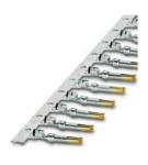
Crimp contact, Socket, rolled, Taped articles, number of pieces per reel: 10000, contact diameter: 1 mm, crimp range:  $0.08~\text{mm}^2$  ...  $0.22~\text{mm}^2$
