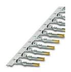
Crimp contact, Socket, rolled, Taped articles, number of pieces per reel: 500, contact diameter: 1 mm, crimp range: 0.08  $\rm mm^2 \dots 0.22~mm^2$
