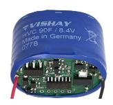
This version is optimized for a 196 HVC in a 90 F, 8.4 V configuration. Basically, it is a voltage converter and switch logic in one, which adjusts to a wide input voltage range. It provides the correct charging voltage and protects against deep discharge.
