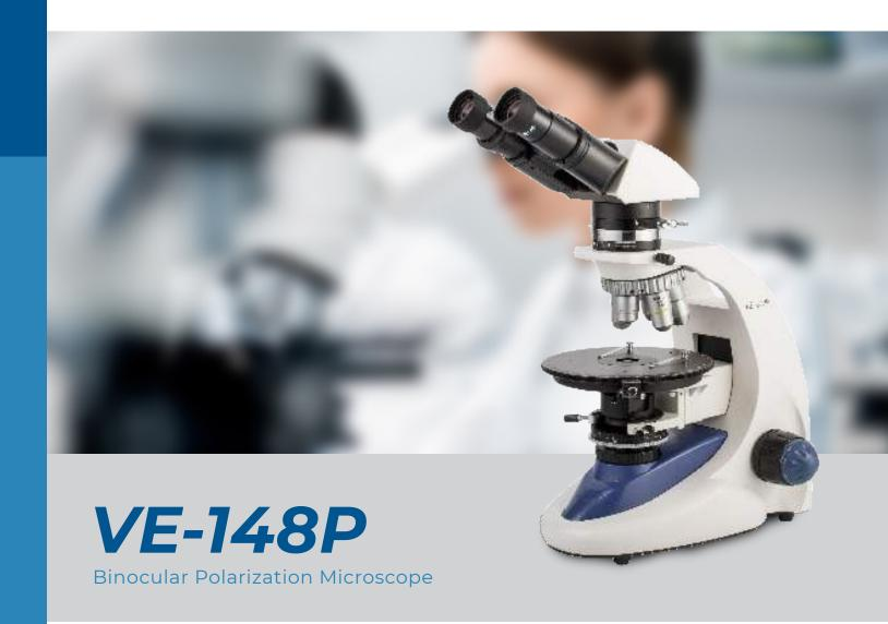
The VE-148P is a professional polarized light microscope, ideal for observing crystalline or fibrous materials and the identification or study of mineral textures. The VE-148P offers observations with 3 types of polarized light (conoscopic, simple and orthogonal) and has a rotating circular stage, divided by a 360° scale.
