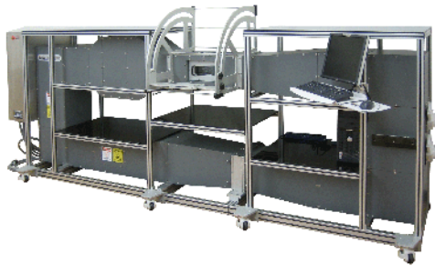
Fig F: FDK Original Wind Tunnel
