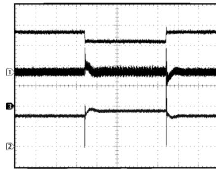
Time Base: 200 \mu s/div V_{OUT} = 5 V I_{OUT} = 500 mA Ch 1: V_{OUT} (5 V/div) Ch 2: I_L + I_{IN} (500 mA/div) Ch 3 (Top Trace): V_{IN} (1 V/div)
