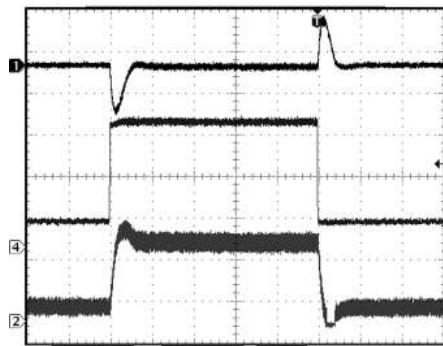
Time Base: 40 \mu s/div V_{IN} = 3.6 V V_{OUT} = 5 V Ch 1: V_{OUT} (500 mV/div) Ch 2: I_L (500 mA/div) Ch 4: I_{OUT} (500 mA/div)
