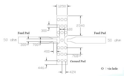
Line width should be designed to match  $50\Omega$  characteristic impedance, depending on PCB material and thickness.
