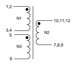
Application of the transformer allows for the leadwires between terminals 1&2, 3&4, 7&8&9, and 10&11&12 to solder bridge.
