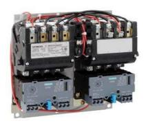
2-speed 3-phase motor starter Size 1 3/4 Two separate windings Constant or variable torque Solid-state overload relays Low SPD OLR range 5.5-22A High SPD OLR range 10-40a 110-120/220-240VAC 60HZ coil Enclosure NEMA type (open) No enclosure
