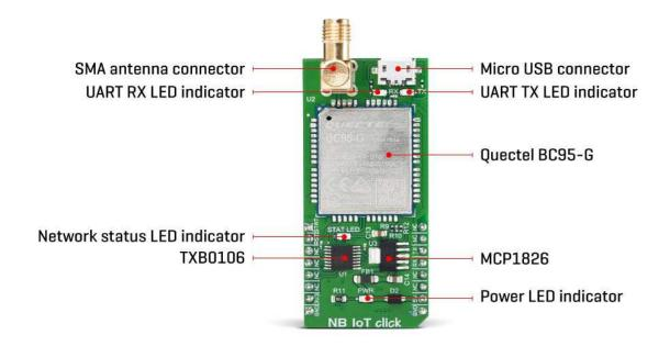
As mentioned before, BC95-G module is the main component of the click board and it consists of a number of internal blocks or sections, such as the RF Transceiver section, Flash SRAM section, Power Management section, and the cellular baseband processor with the peripheral interfaces. BC95 module supports several peripheral interfaces, including two UART interfaces (including the main UART and debug UART interface), USIM card interface, and GPIO interface.
