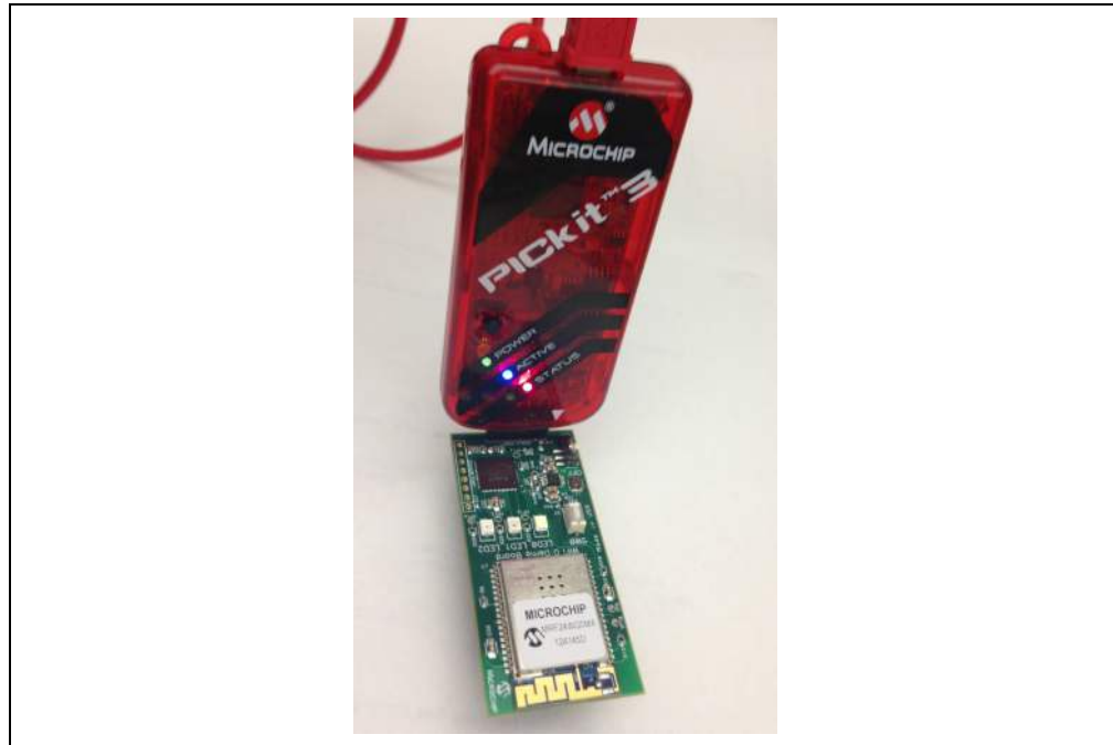
FIGURE 5-3: Wi-Fi® G DEMO BOARD – PICKit™ 3 HARDWARE INTERFACE
