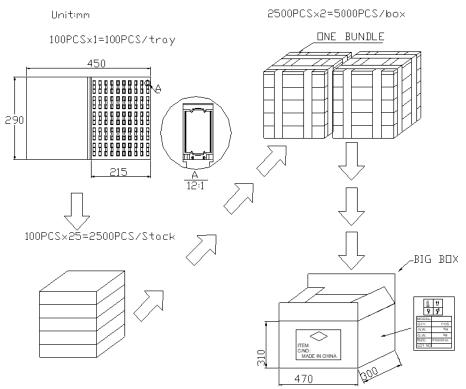
Unless otherwise specified, tolerance: ±10(unit:mm)
