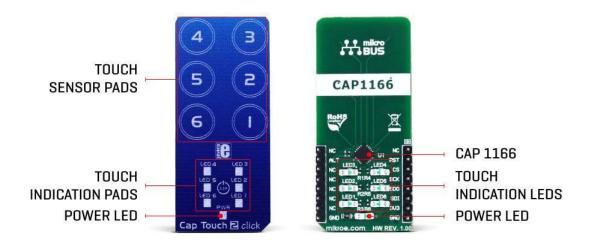
The click board itself has six PCB pads, used to sense touch or proximity events. These pads are the only elements on the top of the board, allowing installation of the protective acrylic glass layer. These pads can be programmed to generate a touch event for both
