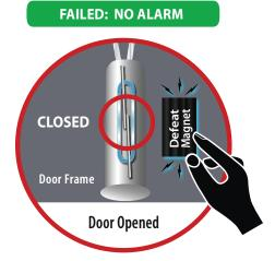
Reed switch contacts are globally magnetic: they will respond to the strongest magnetic field anywhere around the contact -- not solely to the door magnet. When compromised, reed contacts will still send secure signals.
