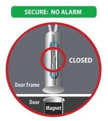
Reed contacts operate on magnetic fields. Most contacts are Closed in the secure position (Closed Loop) when the door is closed and the magnet is near the switch.
