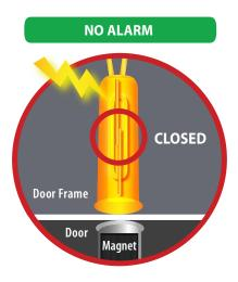
When closed reed contacts are exposed to power surges such as lightning strikes, they are prone to permanent contact welding.
