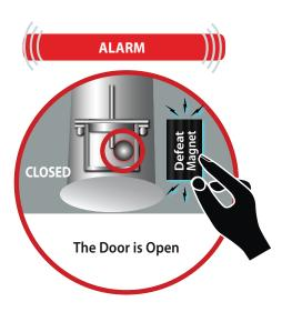
MAGNASPHERE's contact is a spherical magnet and operates in a defined activation zone directed toward the door magnet.
