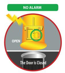
MAGNASPHERE Security Sensors are Open Loop and highly resistant to contact welding from power surges and lightning strikes.
