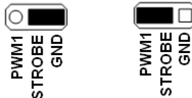
Figure 3. STROBE Jumper Settings
