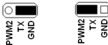
Figure 5. TX Jumper Settings
