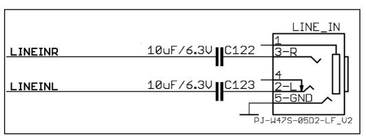
The socket can interface standard 3.5 mm phone connector (also known stereo plug or audio plug).
