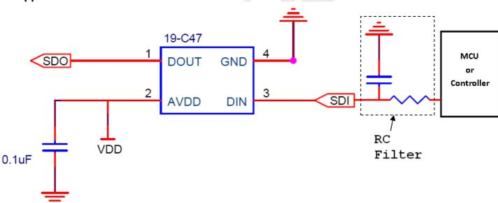
When EAST1818RGBICA0 is set to operate on 5V power system, a 0.1uF capacitor is recommended to add between power supply and ground terminal. The capacitor is suggested to put as closer as possible to IC position. There are frequent resistors were used on different drain voltage as listed table.
