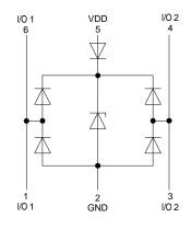
Flow-Thru Design:Route the data lines straight away under the TVS diode I/O pins, that the data signal will not pass through the diode.
