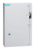
Non-reversing motor starter, Size 4, Three phase full voltage, Solid-state overload relay, OLR amp range 50-200A, 24VAC 50-60Hz coil, Combination type, 200A fusible disconnect, 200A/250V fuse clip, Enclosure NEMA type 1, Indoor general purpose use, Standard width enclosure
