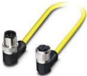
Sensor/Actuator cable, 3-position, TPE, Plug angled M12 SPEEDCON, A-coded, on Socket angled M12 SPEEDCON, A-coded, Cable length: 5 m
