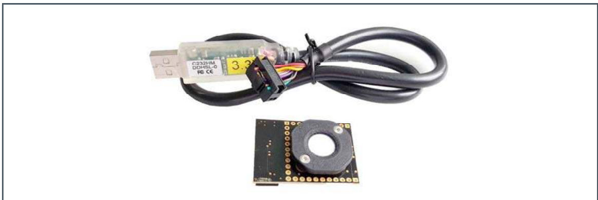
Figure 2: AS7341 Eval Kit with Sensor and Evaluation Board and Pre-Mounted Diffuser
