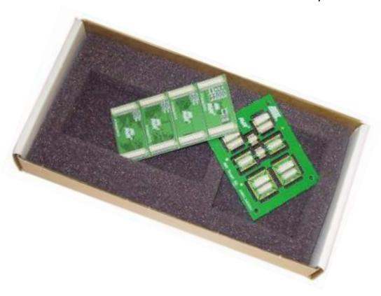
The AVR SMD Emulator Adapter Kit used together with the ICE200 In-Circuit Emulator constitutes an excellent low-cost solution for emulating SMD versions of the AVR® microcontroller family. The kit contains the following features:
