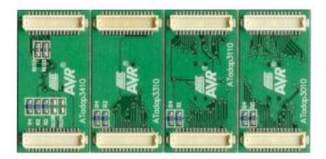
The kit contains two 44-pin TQFP adapters, two 8-pin SOIC adapters, two 20-pin SOIC adapters and two 44-pin PLCC adapters.
