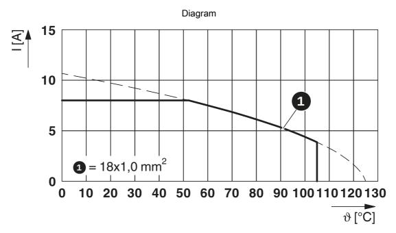
I = current strength,  $\vartheta$  = ambient temperature, 18x 8 A
