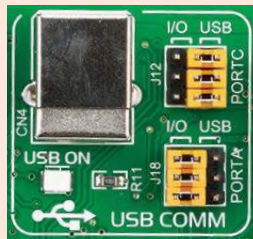
Figure 8-2: USB enabled on PORTC
