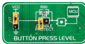
Figure 10-5: Button press level jumper (J17)
