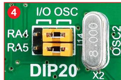
Figure 4-9: RA4 and RA5 connected to X2 quartz-crystal
