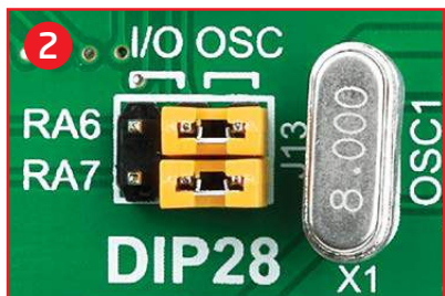
Figure 4-7: RA6 and RA7 connected to X1 quartz-crystal
