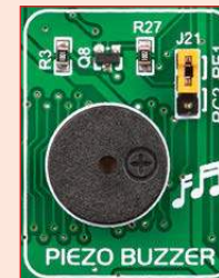
Figure 19-2: Use jumper J21 to connect Piezo buzzer on RE1 or RC2 pin
