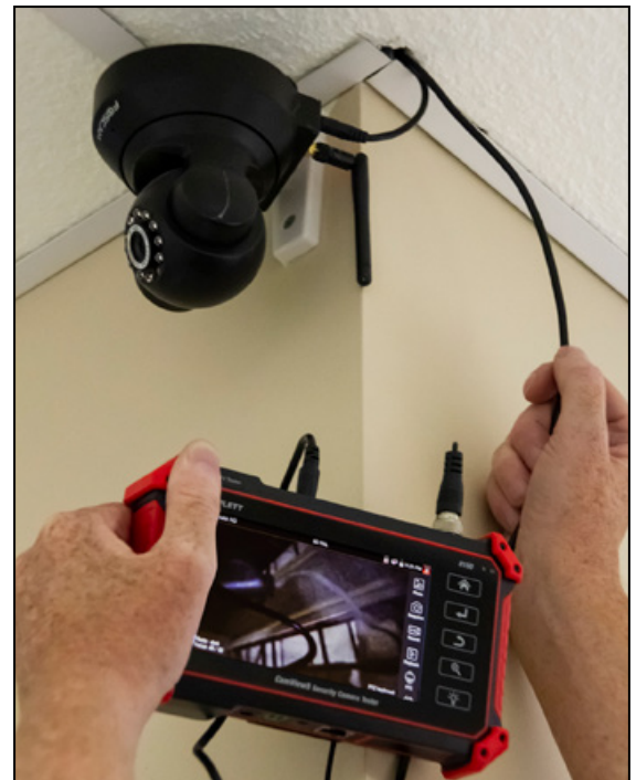
SBR2M Shown here with optional Triplet Model 8150 CamView5 Security Camera Tester
