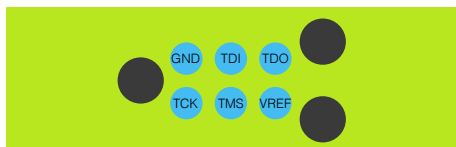
Figure 51: Foot print for tag-connect header
