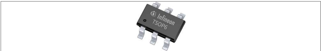
Figure 1-1 Image of TLE4966V in the PG-TSOP6-6-9 package
