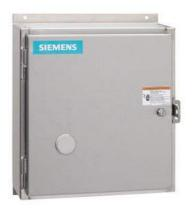
Mechanically held lighting contactor, Contactor amp rating 20Amp 0NC  $\_2NO$  poles, 110-120V 50/60HZ coil, Non-combination type, Encl NEMA type 4X 304 S-steel Water/dust tight noncorrosive
