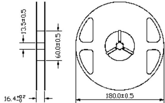
Dimensions of Tape (Unit: mm)
