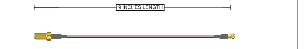
Connector A 132117RP SMA Jack Straight Brass Gold + Heatshrink 50 Ohm RG-316 Continuity/Hi-Pot Connector B 262121 MMCX Jack Straight Bulkhead - Rear Mount Brass Gold + Heatshrink
