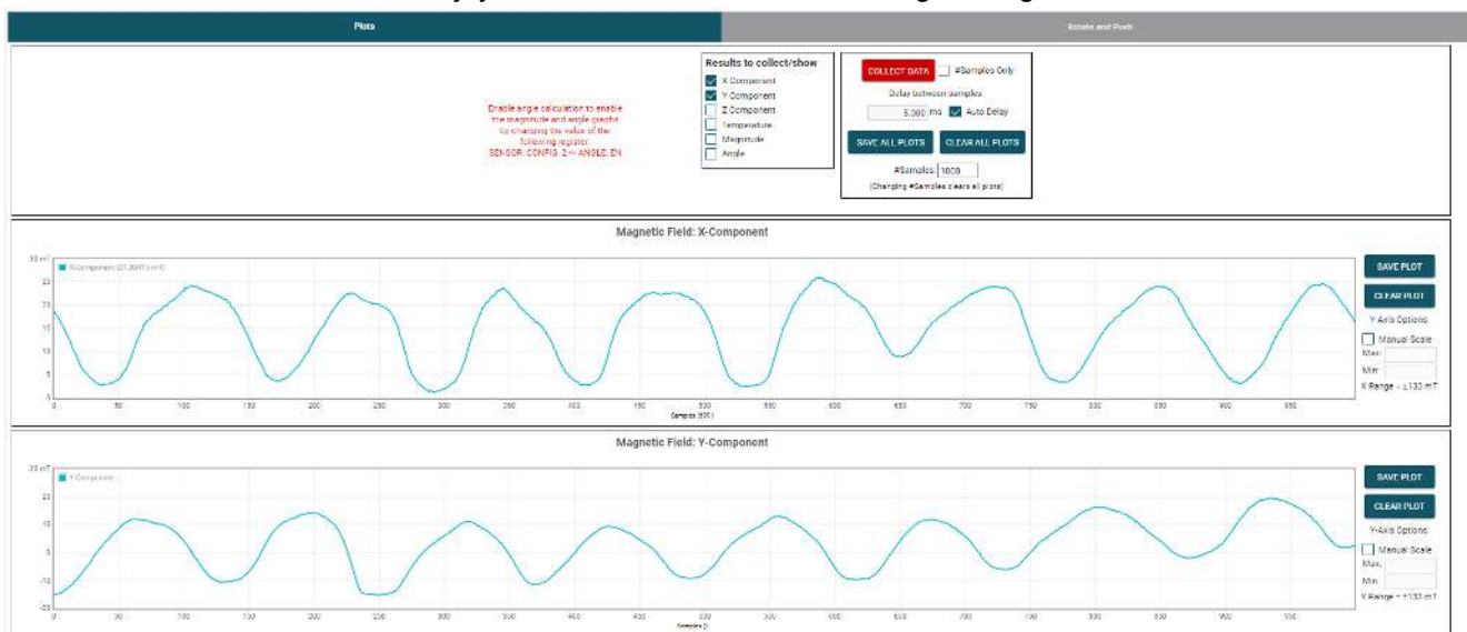
Figure 4-17. Example X and Y Channel GUI Plots After Joystick Movement
