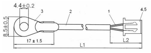
$L1:330\pm10$  Dimensions in mm, Tolerances acc. to ISO 2768-m unless specified
