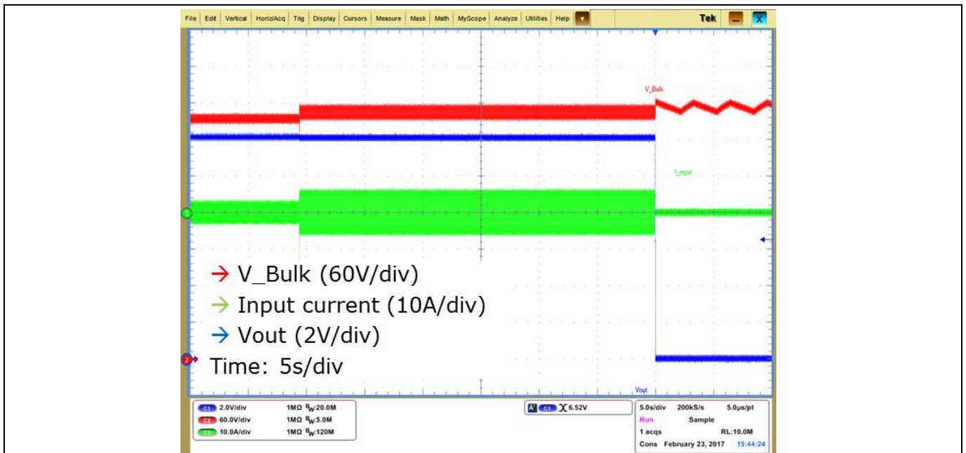
Figure 64 OCP triggered after 30 s with 72 A. Step from half-load.
