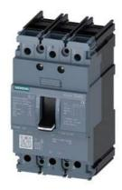
circuit breaker 3VA5 UL frame 125 breaking capacity class S 25kA @ 480 V 3-pole, line protection TM210, FTFM, In=30A overload protection Ir=30A fixed short-circuit protection Ii=10 x In nut keeper kit on both sides
