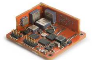
MTi OEM: 37x33x12 mm, 11g, 16-pins header
