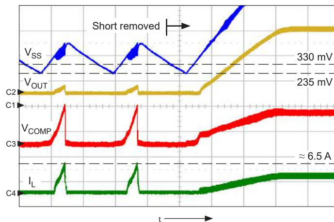
Figure 9. Hiccup mode operation and recovery ; shows V_{SS} (ch1, 200 mV/div.), V_{OUT} (ch2, 2 V/div.), V_{COMP} (ch3, 1 V/div.), I_L (ch4, 5 A/div.), t = 500 \mu s/div.
