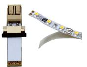
4 Insert flex strip into gap between black sliding latch and beige bridge piece.
