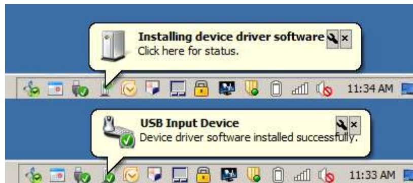
Figure 3-10. Typical Response After Connecting OPTEVM to the Computer
