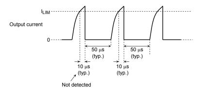
The over-current threshold is a target spec. It varies in a range from approximately 1.5 A to 3.5 A.
