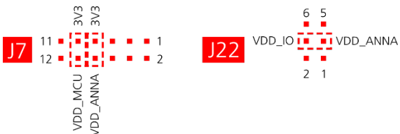
Figure 11: Optional jumper positions while using an external power supply
