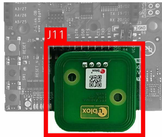
Figure 3: Left: EVB ANNA-B112U including NFC antenna; Right: EVB ANNA-B112U including NFC antenna, turned 180 degrees. Both options are valid.
