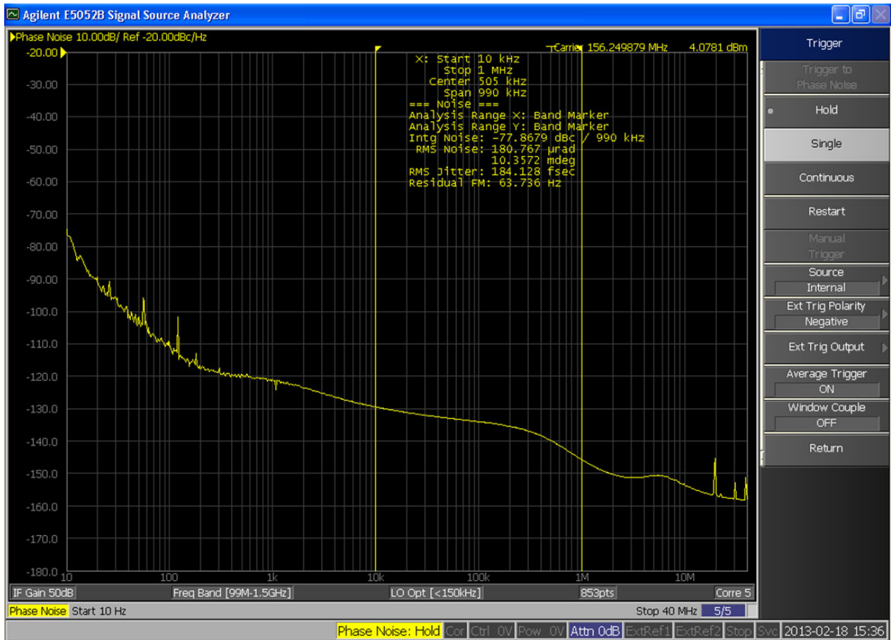
Figure 1. Si535/536 Typical Phase Noise at 156.25 MHz
