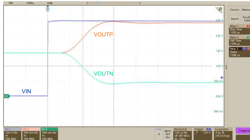
Figure 8-4. Step Response of the AMC1351
