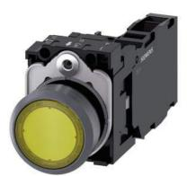
Illuminated pushbutton, 22 mm, round, plastic with metal front ring, yellow, pushbutton, flat, momentary contact type, with holder, 1 NO+1 NC, LED module with integrated LED 230 V AC, screw terminal
