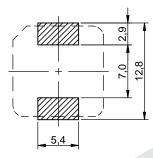
no sensitive traces underneath the component
