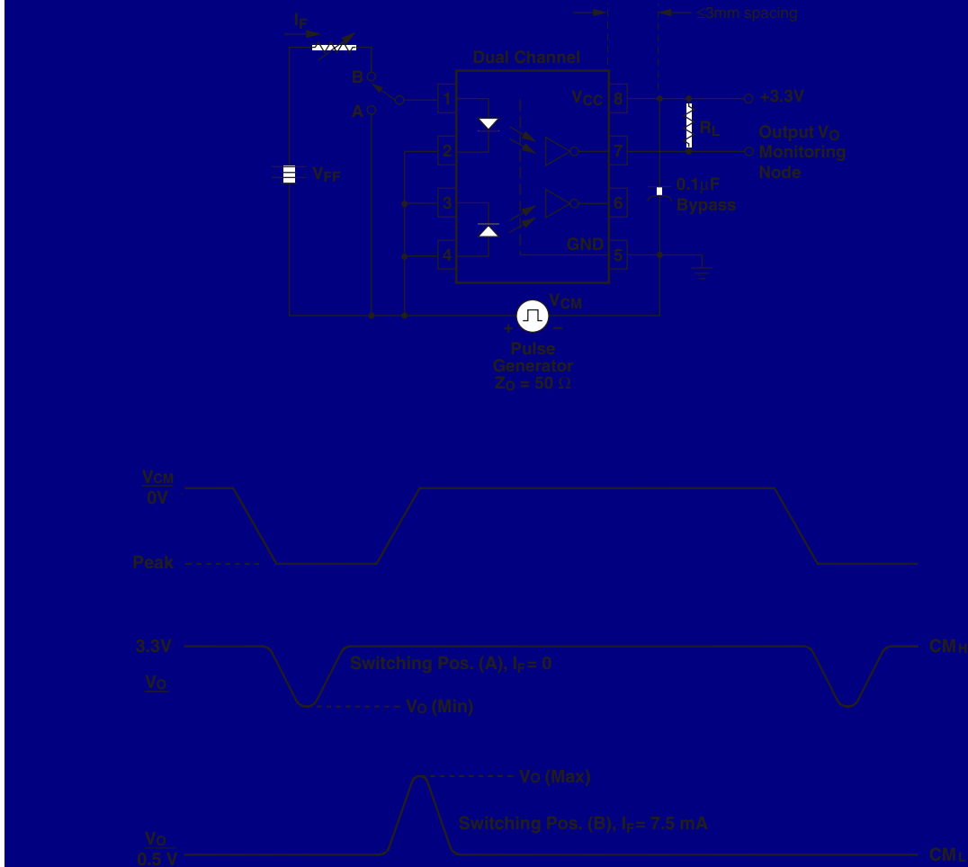
Fig. 11 Test Circuit and Waveforms for Common Mode Transient Immunity
