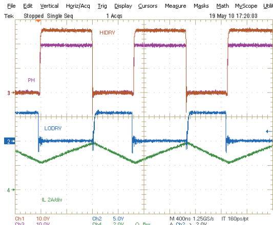
CH1: HIDRV, 10V/div, CH2: LODRV, 5V/div, CH3: PHASE, 10V/div, CH4: inductor current, 2A/div, 400ns/div
