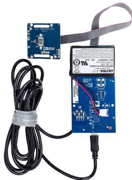
Figure 5. Connect the EVAL-ADPDCUZ to the EVAL-ADPD4200Z-PPG
