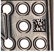
Figure 5: Example Data Matrix Code for Device Identification
