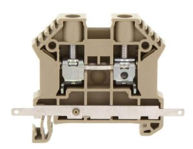
Feed-through terminal, Screw connection, Mounting type: Mounting rail TS 35/7.5, Rated cross-section: 10 mm², Width: 8 mm, Colour: White
