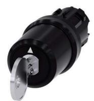
key-operated switch Siemens, 22 mm, round, plastic, lock number SSG10, with 2 keys, 3 switch positions I-O-II, latching, actuating angle 2x45°, 10:30h/12h/13:30h, key removal I+O+II, with laser labeling, inscription or symbol customer-specific selection with SIRIUS ACT configurator (CIN)
